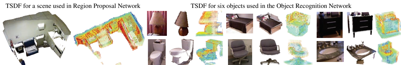
Figure 3. Visualization of TSDF Encoding. We only visualize the TSDF values when close to the surface. Red indicates the voxel is in front of surfaces; and blue indicates the voxel is behind the surface. The resolution is 208 \times 208 \times 100 for the Region Proposal Network, and 30 \times 30 \times 30 for the Object Recognition Network.
